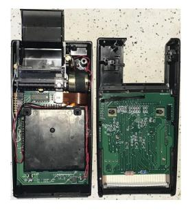
Align the case halves so that the latch on the top half engages under the lip on the lower case half.
