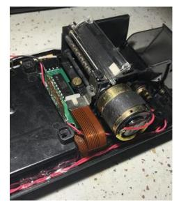
Carefully insert the ribbon cable into the socket on the battery board. The tool described above can help with this procedure.
