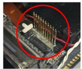
To fit them so that they line up properly, the CPU board needs to be placed onto the pins that were just soldered. The CPU board should be parallel to the battery board after assembly.
