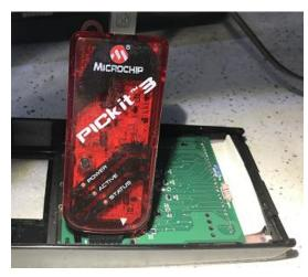
The PICkit3 can be plugged into the holes on the circuit board using the 6 pin IDC connector as shown
