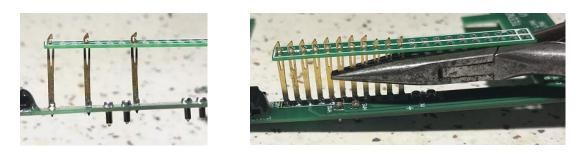
Once you are happy with the positioning, insert a few other long pins, but make sure you leave the right most three holes free for the shorter pins. As you add the pins, you can use the template board to hold them in place and use pliers as shown to make sure the pins are aligned.
